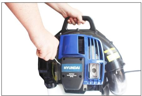
4. When the machine starts, move the Choke Lever down in to the "Run Position". YOU MUST do this step, as the machine will over fuel and stop.
